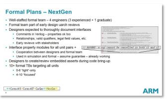
Formal experts enabling designers to use FV, with focus on properties that are hard to verify with simulation
