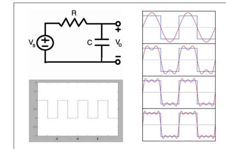
If the source voltage  $V_S$  is sinusoidal, the impedance  $Z_C$  of the capacitor is constant.
